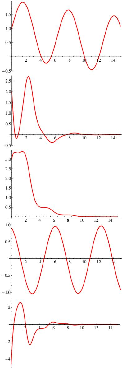
Fig. 1. Simulations of Chain of Integrators (38) Tracking  $(\sin(t), 0, 0)^\top$  with our Closed Loop Control, Initial Function  $\xi_0 = (1, 2, 3)^\top$ , Delay  $\tau = 1/6$  and  $a_0 = 1/(4\pi)$ . Top to Bottom:  $\xi_1(t)$ ,  $\xi_2(t)$ ,  $\xi_3(t)$ ,  $v_1(t)$ , and  $v_2(t)$ .
